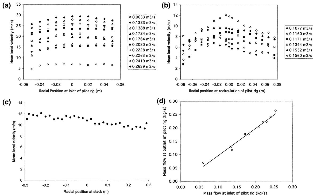
**Figure 5.** Velocity profiles: (a) inlet to pilot-scale cyclones, (b) recirculation to pilot-scale cyclones, and (c) stack. (d) Gas mass balances (pilot-scale).
