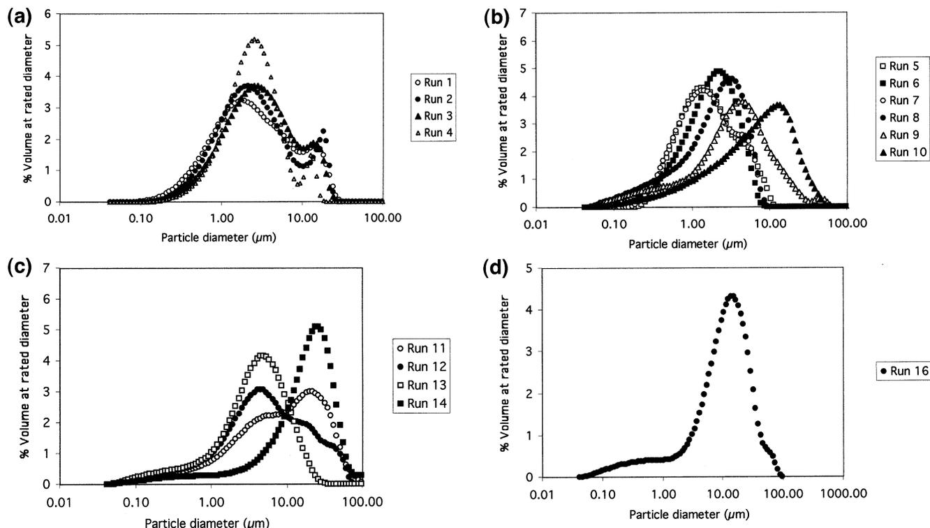
**Figure 11.** Outlet distributions from (a) the pilot-scale RS\_VHE cyclone, (b) the recirculation system, (c) the pilot-scale HE cyclone, and (d) the pulse jet bag filter.
