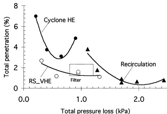
**Figure 8.** Global collection (pilot-scale cyclones and filter).
