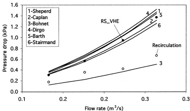
**Figure 6.** Pressure drop (pilot-scale RS\_VHE and concentrator).
