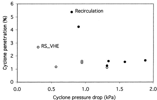
**Figure 9.** Cyclone in-loop penetration.
