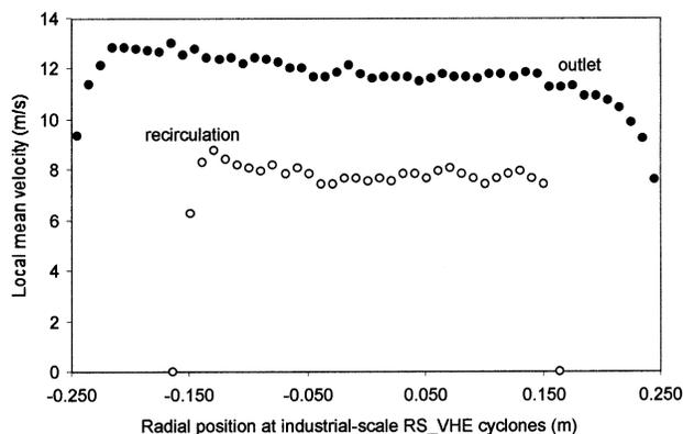
**Figure 13.** Velocity traverse at the outlet of the industrial-scale RS\_VHE and recirculation cyclones.
