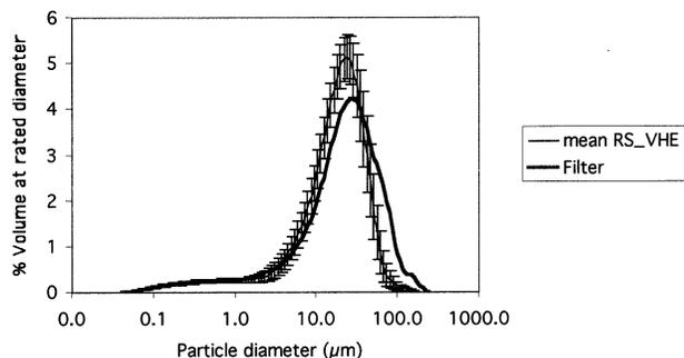
**Figure 7.** Inlet distribution to the pilot-scale cyclones and bag filter.
