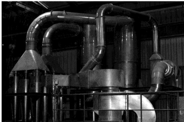
**Figure 12.** Industrial-scale RS\_VHE and recirculation cyclones.
