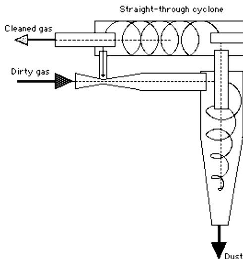
**Figure 3.** Proposed collector-first recirculation system.
