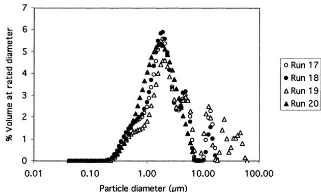
**Figure 15.** Size distributions (industrial recirculation system).
