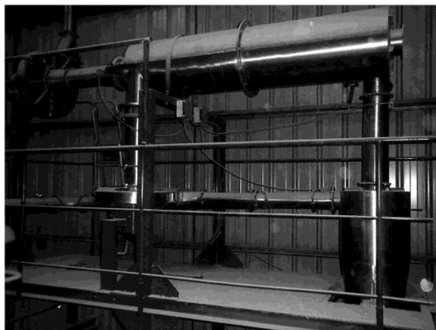
**Figure 4.** Pilot-scale system (RS\_VHE cyclone and concentrator).
