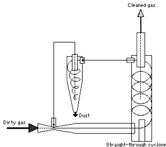
Figure 2. Concentrator-first recirculation system.
