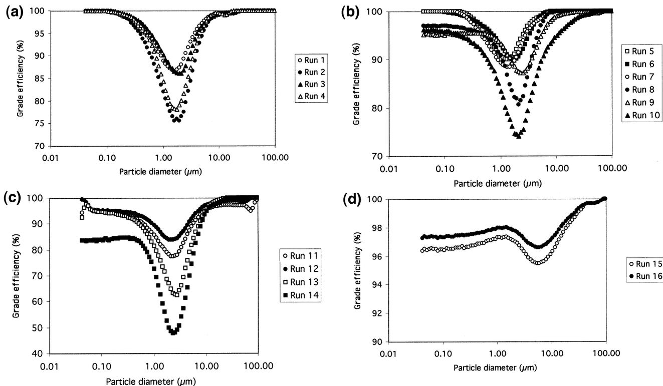
**Figure 10.** Grade efficiencies of (a) the pilot-scale RS\_VHE cyclone, (b) the recirculation system, (c) the pilot-scale HE cyclone, and (d) the pulse jet bag filter.
