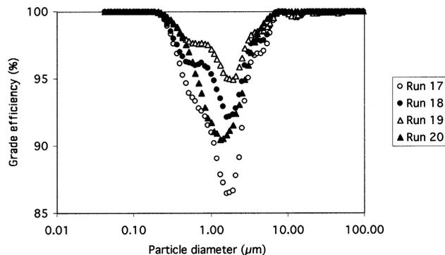
**Figure 14.** Grade efficiencies (industrial recirculation system).
