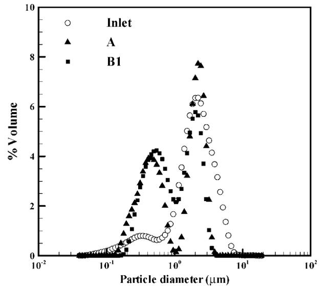
**Figure 6.** Particle size distributions at the inlet (average) and at the outlet for the two recirculating cyclone systems (A: RS\_VHE 2 system,  $226 \text{ mg} \cdot \text{m}^{-3}$  at STP,  $4.0 \times 10^{-4} \text{ m}^3 \cdot \text{s}^{-1}$  at STP; B1: RS\_VHE 2.6 system,  $221 \text{ mg} \cdot \text{m}^{-3}$  at STP,  $2.9 \times 10^{-4} \text{ m}^3 \cdot \text{s}^{-1}$  at STP).
