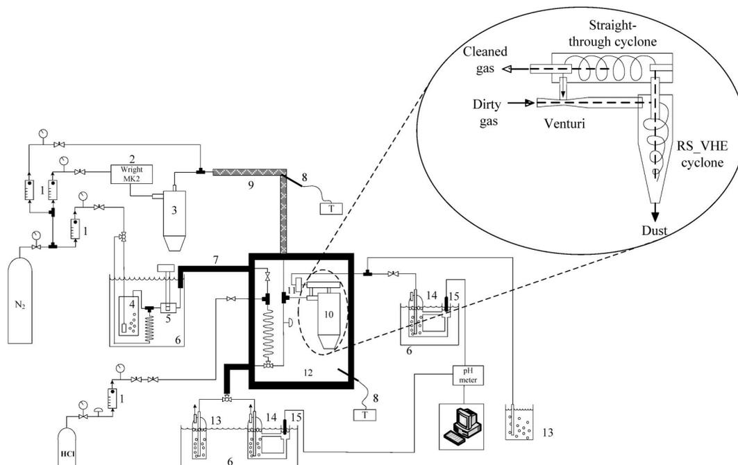
(⊖) manometer; (⊕) pressure regulator; (⊖) on/off valve; (⊗) needle valve; (⊗) three-way valve; (⊗) check valve. 1: rotameter; 2: solid particles feeder; 3: deagglomerating cyclone; 4: humidification column; 5: hygrometer; 6: temperature controlled bath; 7: thermal insulation; 8: thermocouple; 9: electrical heating tape; 10: cyclone reactor; 11: filter; 12: oven; 13: absorber; 14: absorber with lateral chamber; 15: pH electrode.
