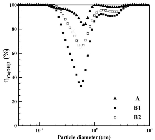
**Figure 7.** Grade efficiency curves for the capture of  $\text{Ca(OH)}_2$  particles (A: RS\_VHE 2 system,  $226 \text{ mg} \cdot \text{m}^{-3}$  at STP; B1: RS\_VHE 2.6 system,  $221 \text{ mg} \cdot \text{m}^{-3}$  at STP; B2: RS\_VHE 2.6 system,  $683 \text{ mg} \cdot \text{m}^{-3}$  at STP).
