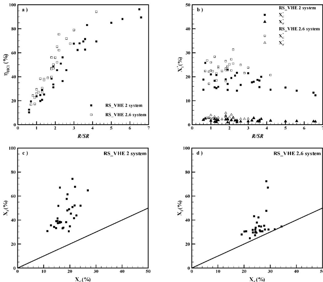
Figure 3. Experimental results for the acid gas removal efficiency (a), for the solid reactant's conversion relative to the fresh feed (b) and for the solid reactant's conversion relative to the captured sample (c and d) for the two recirculating cyclone systems tested. The solid line is filter conversion if equal to cyclone conversion ( $X_c$ ).
