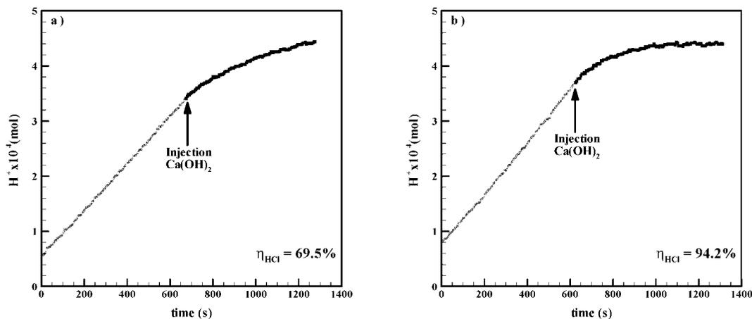
Figure 2. Experimental variation of  $H^+$  vs time ( $R/SR = 4.2$ ). (a) RS\_VHE 2 system,  $C_{HCl} = 1.10 \times 10^{-2} \text{ mol} \cdot \text{m}^{-3}$ . (b) RS\_VHE 2.6 system,  $C_{HCl} = 1.20 \times 10^{-2} \text{ mol} \cdot \text{m}^{-3}$ .
