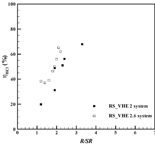
**Figure 5.** Experimental results for acid gas removal varying the acid gas concentration and  $W_{\text{Ca(OH)}_2} = (3.1 \pm 0.3) \times 10^{-7} \text{ kg} \cdot \text{s}^{-1}$ .
