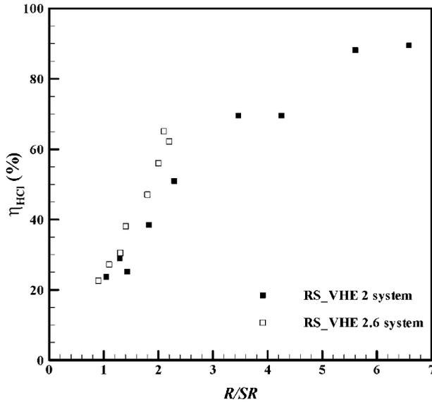
**Figure 4.** Experimental results for acid gas removal varying the fresh solid reactant's feed rate and  $C_{\text{HCl}} = (1.0 \pm 0.1) \times 10^{-2} \text{ mol} \cdot \text{m}^{-3}$ .
