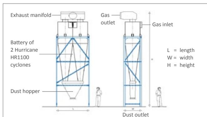
Fig.5 – General arrangement of the Hurricane cyclone system
