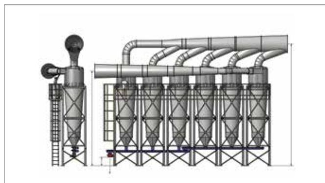
Fig. 6 – System composed by 6 Hurricane HR numerically optimized cyclones, with ø1550mm
