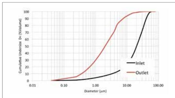
Fig. 3 – Particle size distribution used in simulation
