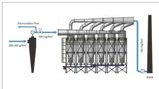
Fig.5 – General arrangement of the Hurricane cyclone system
